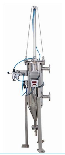
Disc Type Self Cleaning Filter is used for highly viscous material filtration like Greece, Lube Oil, Edible Oil, Toothpaste & many more. Here, we don't required any backwashing media to clean the Filter Element. It is working under principle of differential pressure parameters for uninterrupted filtration requirement.
