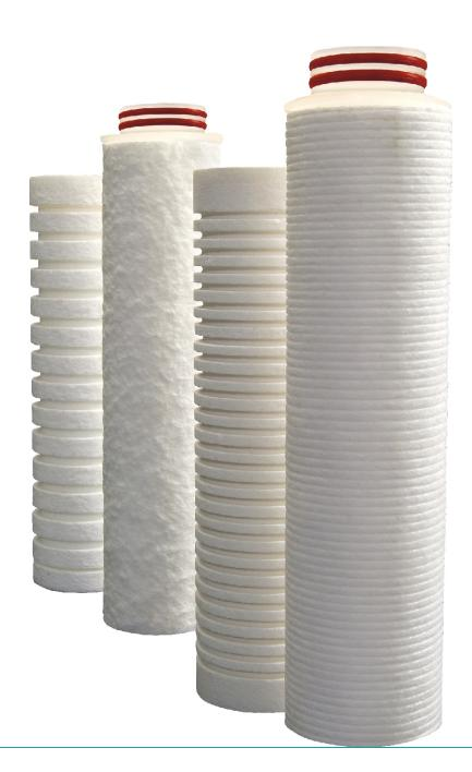
Spun bonded filter cartridges are made up of 100% polypropylene fibers. The fibers have been carefully spun together to form a true gradient density from outer to inner surface. Filter cartridges are available with core & without core version. The superior structure remains integral even under severe operating conditions and there is no media migration. Polypropylene fibers are blown continuously on central molded core, without any binders, resins or lubricants.
