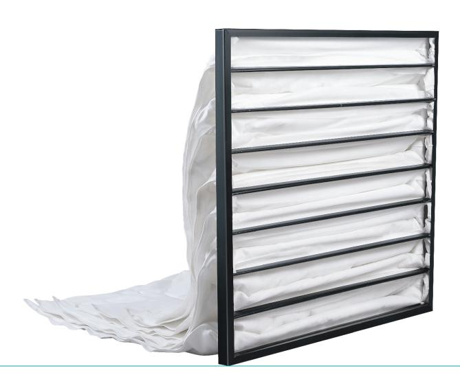
Pocket filter are made up of non woven synthetic fiber media to ensure retention of solid particles up to the stipulated micron rating. These are covered with supporting layer of spun bonded media to avoid any type of particles or fiber migration, even after high pressure build up. Media are sealed with thermal bonding or stitching as per requirement.
