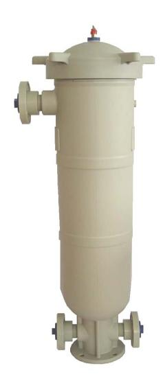
Plastic Bag Housing is made of 100% pure German made Polypropylene resin, by integrated one-piece injection molding technologies, featuring excellent resistance to pressure, corrosion and ultraviolet light attack. It is designed to use industrial standard Size two filter bags (Ø 7" X 32"long); Filter Housing has broad applications, and is ideal for high flow, corrosive and outdoor applications.
